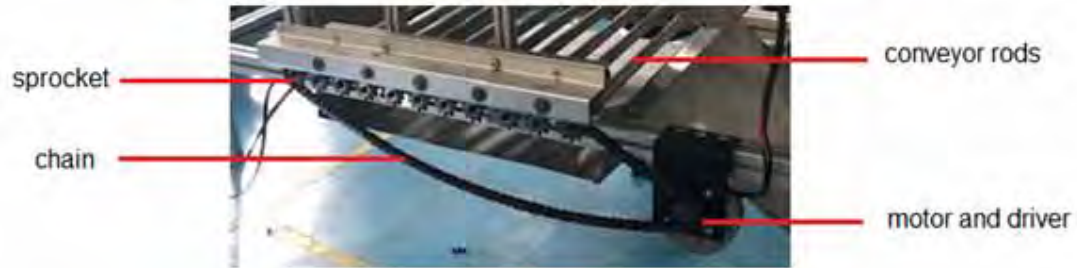
Figure 4.2 Closed-up the completed conveyor set with sprocket, chain, motor and driver
